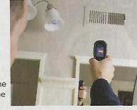
ergonomic and pocket portable so it is always available for instant troubleshooting. Simply aim the instrument at a target object or surface to measure the temperature, then click the trigger to freeze and view the image.
